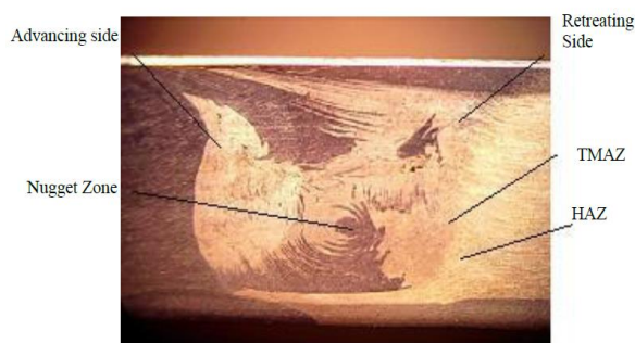
Figure 12. Macrograph of cross section of welded sample.
